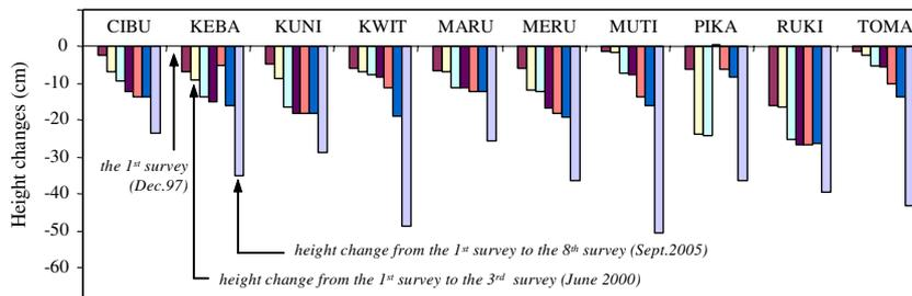
**Fig. 7** Accumulated GPS-derived subsidence (cm) during the period of June 2001–September 2005
