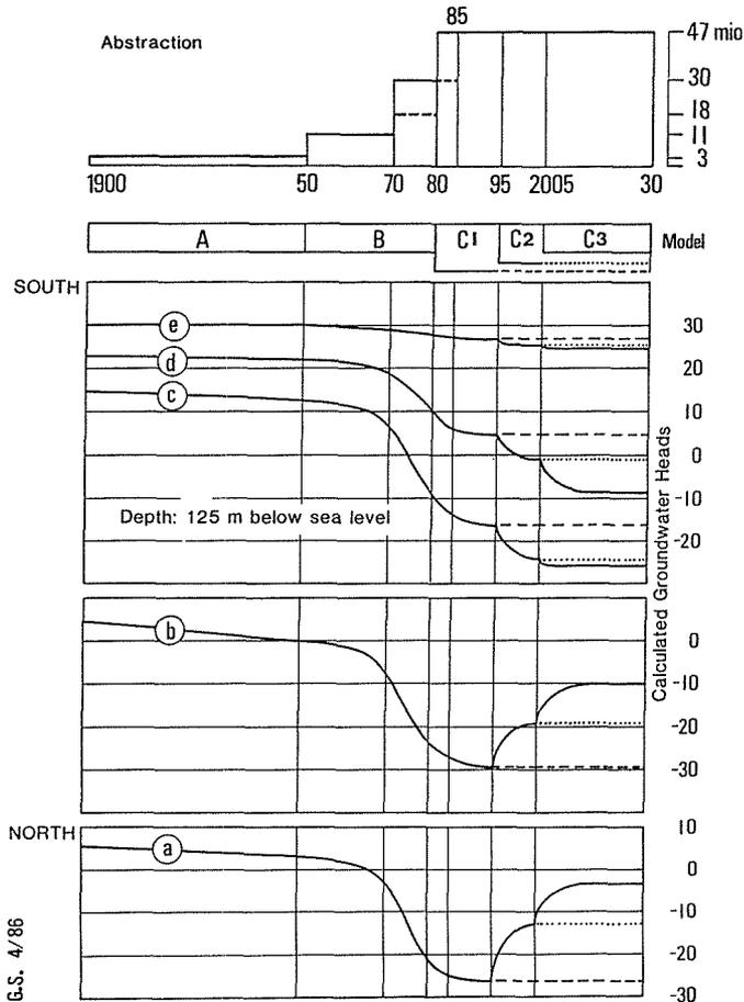
Figure 6. Development of piezometric heads at selected reference nodes of the model for the abstraction configurations A, B and C1, C2, C3; aquifer depth 125 m.
