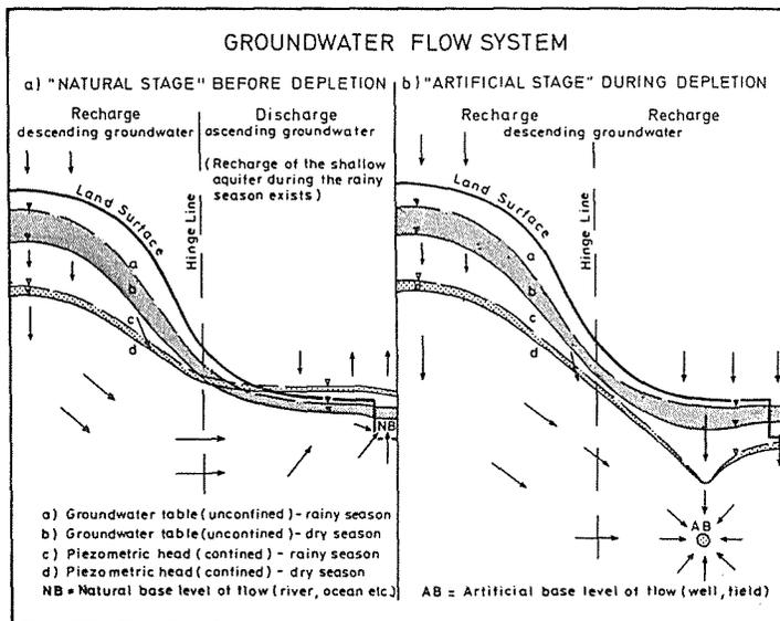
Figure 3. Principles of groundwater flow in the Jakarta area before and during over-exploitation.
