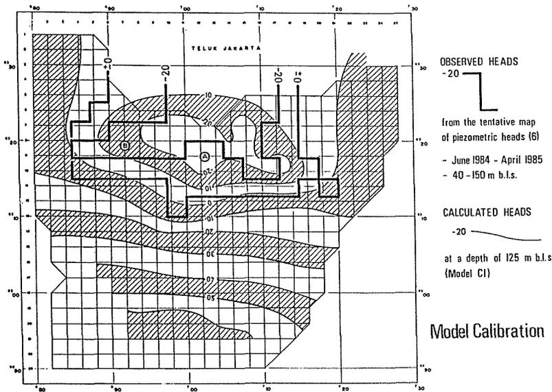
Figure 2. Isolines of observed and calculated piezometric heads, 1984/85, aquifer depths 40-150 m.
